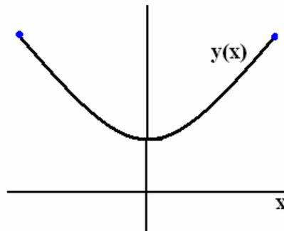
Fig. 1 Heavy cord fixed at its ends
